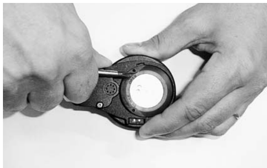
Fig. 5.3. Opening of securing ring.
