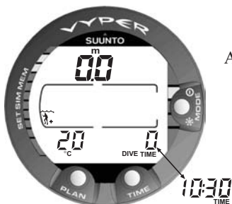
Fig 3.4 Startup IV. The Surface Mode: The depth and dive time are zeros (as no dives have yet been made), and the temperature is 20°C [68°F].
