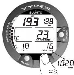
Fig. 3.8 Diving display. The present depth is 19.3 m [63 ft] and the no-decompression time limit is 23 minutes in A0/P1 mode. The maximum depth during this dive was 19.8 m [65 ft], the elapsed dive time is 16 minutes and the water temperature 18°C [64°F]. The current time 10:20 [10:20 am] is shown for 5 seconds after pressing the TIME button.
