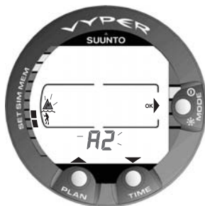
Fig. 4.25 Adjusting The Altitude Setting. Press the scroll buttons to change the altitude mode.
