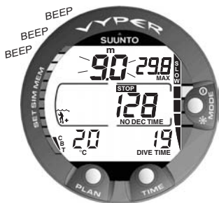
Fig. 3.13 Ascent Rate Indicator. Blinking depth reading, SLOW and four segments shown: ascent rate is more than 10 m/min [33 ft/min]. This is a caution to slow down! The STOP sign means that you are advised to make a Mandatory Safety Stop when you reach the depth of 6 m [20 ft].
