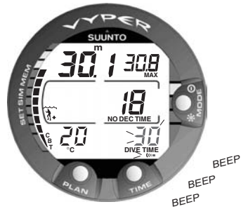
Fig. 3.32 Preset dive time alarm is activated.
