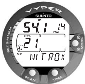
Fig. 3.20 Nitrox display. The maximum depth based on set O_2\% (21%) and PO_2 (1.4 bar) is 54.1 m [177 ft].
