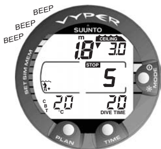
Fig. 3.14 A Mandatory Safety Stop. You are advised to make a Mandatory Safety Stop in the depth zone between 6 m and 3 m [20 ft and 10 ft]. Pressing the TIME button shows the alternative display.
