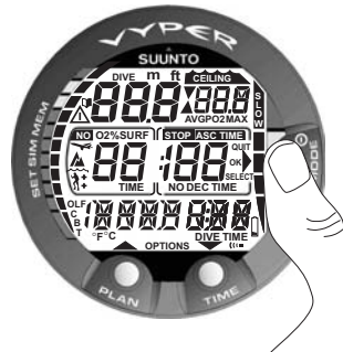
Fig. 3.1 Startup I. All segments shown.
