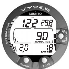
Fig. 3.11 Ascent rate indicator. Three segments.
