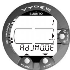
Fig. 4.24 Altitude Adjustment and Personal Adjustment Setting Mode. [1 AdJ MODE].
