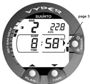
Fig. 4.9 Logbook, page III. The surface interval time and average depth.
