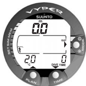
Fig. 4.18 Selected Dive Simulator Mode. Descent by pressing the arrow down (TIME) button and ascent by pressing the arrow up (PLAN) button.
