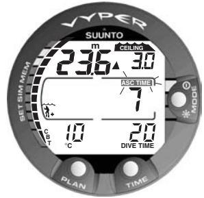
Fig. 3.16 Decompression dive, below the floor. The upward pointing arrow and the blinking ASC TIME label tell you to ascend. The minimum total ascent time including the safety stop is 7 minutes. The ceiling is at 3 m [10 ft].
