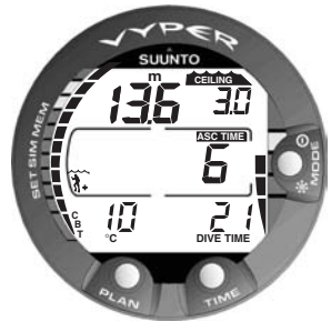
Fig. 3.17 Decompression dive, above the floor. The upward pointing arrow has disappeared and the ASC TIME label has stopped blinking, which means that you are in the decompression range.
