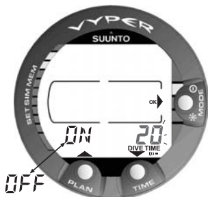
Fig. 4.28 Setting The Dive Time Alarm. Press the scroll buttons to change the alarm on/off and to set the dive time value.
