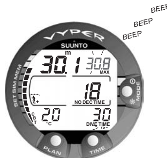
Fig. 3.33 Preset maximum depth alarm is activated.
