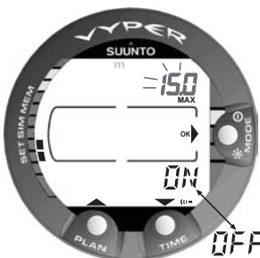
Fig. 4.30 Setting The Maximum Depth Alarm. Press the scroll buttons to change the alarm on/off and to set the maximum depth value.
