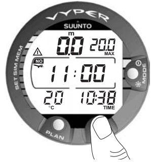
Fig. 3.29 Surface interval, no-flying time. Pressing the TIME button twice will show the no-flying time, indicated by an airplane symbol.
