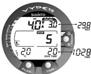
Fig. 3.14 A Mandatory Safety Stop. You are advised to make a Mandatory Safety Stop in the depth zone between 6 m and 3 m [20 ft and 10 ft]. Pressing the TIME button shows the alternative display.
