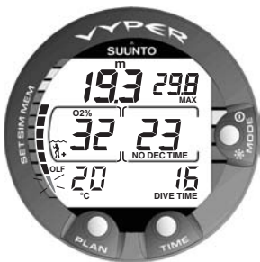
Fig. 3.25 The lowest bar graph blinks to indicate that the OLF value shown relates to OTU.
