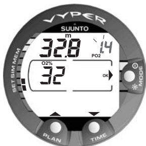
Fig. 4.32 Setting Oxygen Percentage and Partial Pressure. The equivalent maximum depth is 32.8 m [107 ft]. Press the scroll buttons to change the oxygen percentage and to set the oxygen partial setting value.
