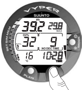
Fig. 3.24 Alternative display. Pressing the TIME button displays the current time, maximum depth and CBT.
