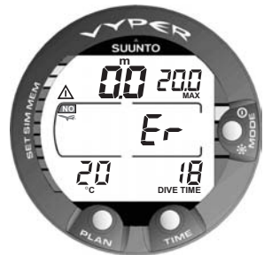
Fig. 3.30 Surface Mode after a violated decompression dive. The Er symbol indicates that you have violated the ceiling for more than three minutes. You must not dive again for at least 48 hours.
