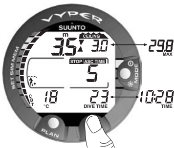
Fig. 3.18 Decompression dive, at the ceiling zone. The two arrows point at each other ("hour glass"). You are at the optimum ceiling zone at 3.5 m [11 ft] and your minimum ascent time is 5 minutes. By pressing the TIME button you can display maximum depth and time.
