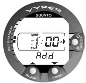
Fig. 4.20 Selected Dive Planning Simulator Mode. Add the desired surface interval increment (to present shown surface interval) by pressing the TIME and PLAN buttons. NOTE! This display is only shown for repetitive dives.
