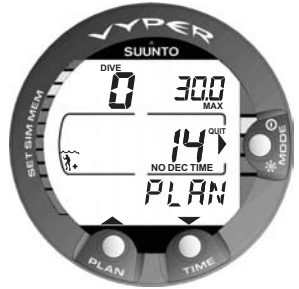
Fig. 3.6 Dive Planning. The Planning mode is indicated by the PLAN text. The no-decompression time limit at 30.0 m [100 ft] is 14 minutes in A0/P1 mode.
