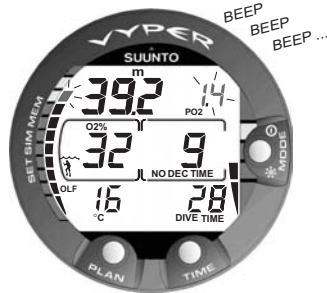
Fig. 3.23 Oxygen partial pressure and OLF displays. There is an audible alarm as the oxygen partial pressure is greater than 1.4 bar or the set value and the OLF has reached the 80% limit.
