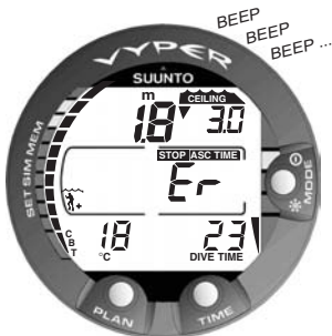
Fig. 3.19 Decompression dive, above ceiling. Note the downward pointing arrow and the Er warning. You will also hear an audible alarm. You should immediately (within 3 minutes) descend to or below the ceiling.
