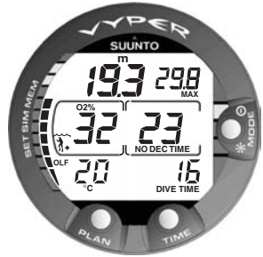
Fig. 3.22 Diving in the NITROX Mode. The O_2\% is set to 32%.
