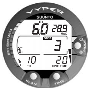
Fig. 3.10 Ascent rate indicator. Two segments.
