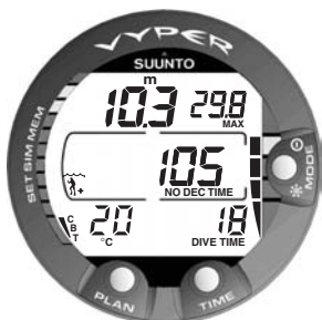
Fig. 3.12 Ascent rate indicator. Four segments.
