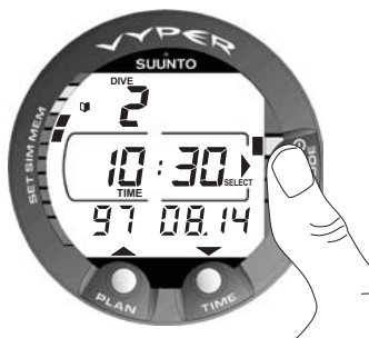
Fig. 4.11 Logbook, page I. Press the SMART (Select) button once to be able to scroll between the different dives.
